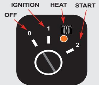
*If the engine fails to start after 10 seconds of cranking, leave for 1 minute and try again.*
